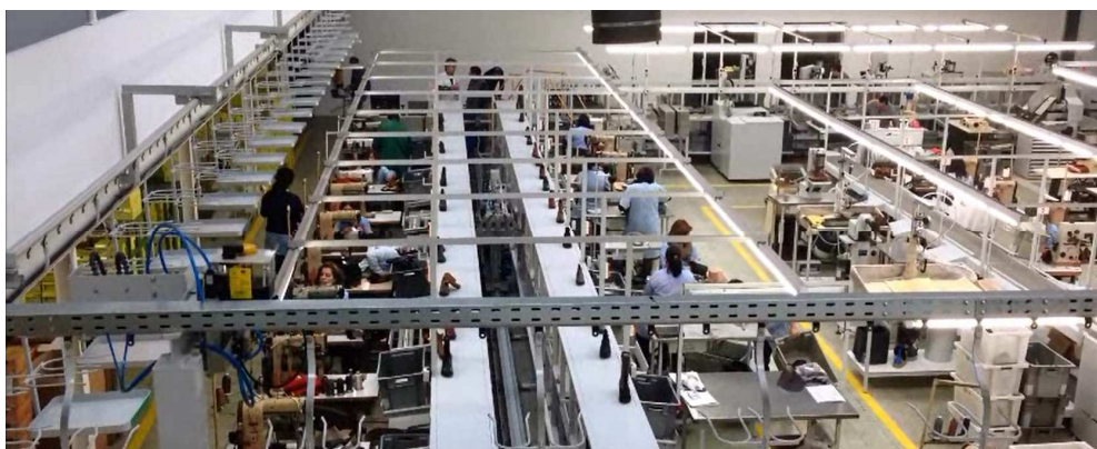
Figure 10 – The High Speed Shoe Factory: stitching production lines
