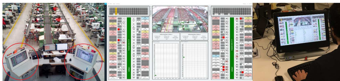
Figure 20 - Working Posts Monitor: on the manufacturing line (left photograph), its display screen (screen shot on the middle) and on the ICT department (right photograph)
